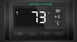
In this mode, the fans will run continuously regardless of temperature or humidity, the speed set in this mode will be the max speed the fans can reach in AUTO Mode.
