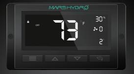
In this mode, the fans will not run regardless of temperature or humidity. While in this mode, pressing the up or down button will change the display's brightness.
